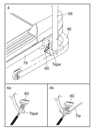
4. Raise the Right Handrail (59) and the Left Handrail (not shown) so the Base (46) is flat on the floor. Next, postition the Handrails near the Frame (79).
